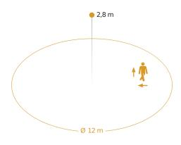
Possible mounting height: 2,50 m - 4,00 m Orange: radial and tangential
